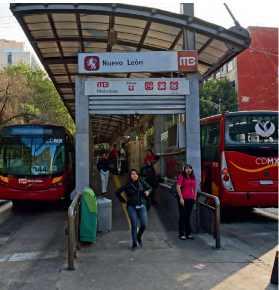
Figure A30. Mexico City BRT uses low-grade transitions between street and station (ITDP, 2022a).
