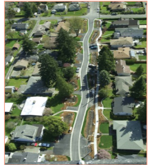
Figure 12. The curvilinear nature of this right of way provides traffic calming effects. 31
